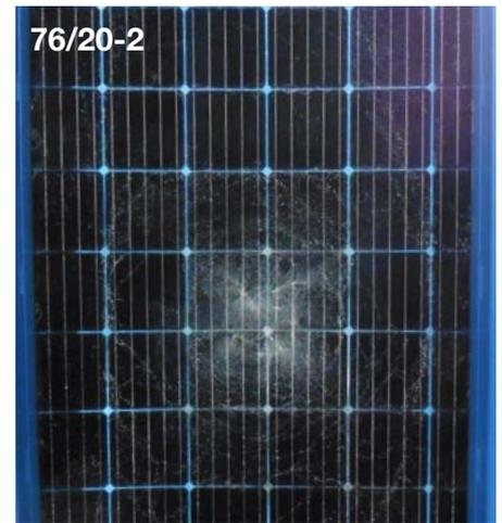
The GridParity modules have passed all tests with excellence. Not a single module was massively damaged or even penetrated as the photos show. The modules may therefore be used for overhead glazing, facade installations and as balcony modules. This results in a wide range of applications from terraces to carports, large-scale parking lot roofing, roofing of industrial halls to sports facility roofing.
