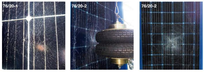
The GridParity modules have passed all tests with excellence. Not a single module was massively damaged or even penetrated as the photos show. The modules may therefore be used for overhead glazing, facade installations and as balcony modules. This results in a wide range of applications from terraces to carports, large-scale parking lot roofing, roofing of industrial halls to sports facility roofing.
